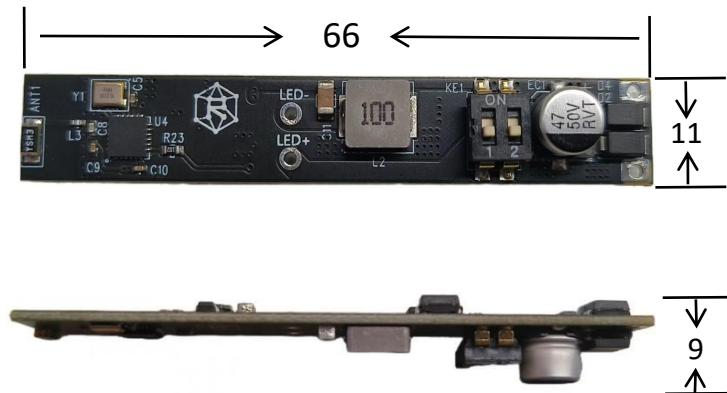
$$A \times B \times C = 66 \times 11 \times 9 \text{ Unit:mm}$$
